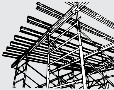
BrandSafway® ALJ Aluminum beams can be used as both joists and stringers.
